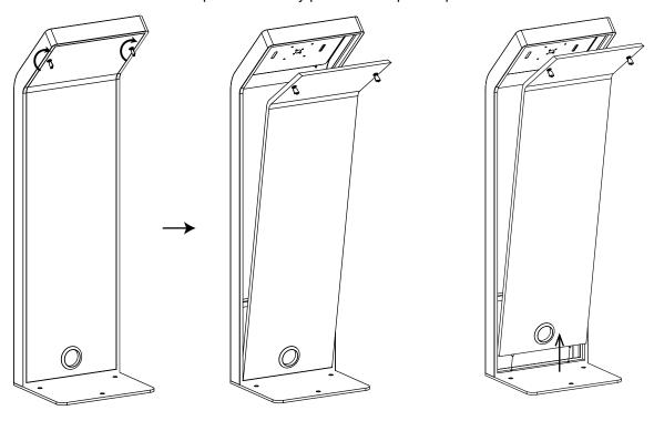
Inside the enclosure, turn the tabs outwards at the top as shown. The tablet holder can be release now.
